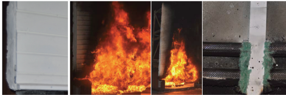
Vented Construction Systems (VCS) assembly (by Teknos, applying Securo FB vented fireblocking) tested at SP Sweden: Image 1 show cladding assembly prior to test. Image 4 show cavity with wooden cladding removed after test: Note backing surface, wood stud fire block, vented fire block and rockwool end seals. The severe direct flame exposure was instantly blocked by the horizontal vented fire block and did not penetrate to air cavity above.
